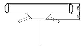
Installation space for reading devices (without passage indicator, mounting depth 40 mm)
