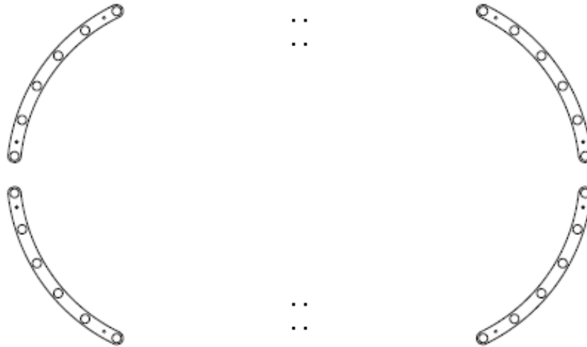
Figure E: Mounting the curved yoke pieces to the concrete.
