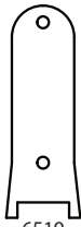
6519 Fail Open Linkage These have an approximate length of 2.5" and do not have the extra hole for the key override option.
